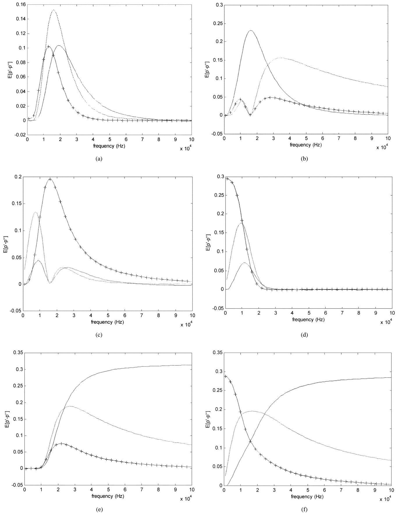
Fig. 2.  $E(|\hat{P}'_\gamma - \hat{P}''_\gamma|)$  function for the different fault classes (“-” for node  $V_a$ , “- -” for  $V_b$ , “+” for node  $V_c$ ). (a) Class 1: R6, R7 faulty; (b) class 2: R3, C1 faulty; (c) class 3: R4, C2 faulty; (d) Class 4: R5 faulty; (e) class 5: R2 faulty; (f) class 6: R1 faulty.
