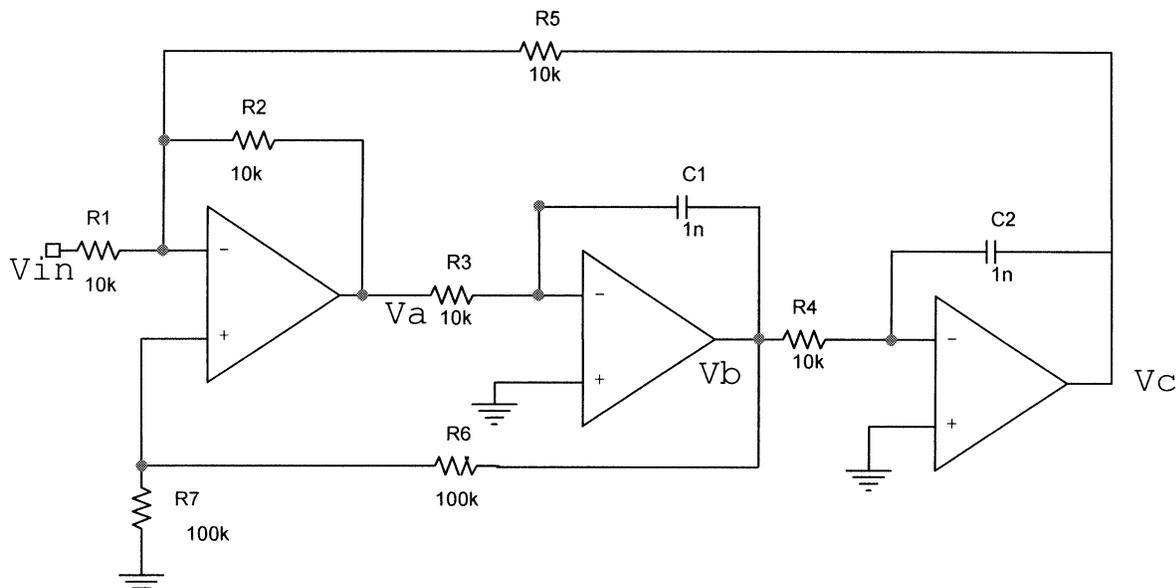
Fig. 1. CUT: a Biquad filter. The nominal values are in the appropriate units.
