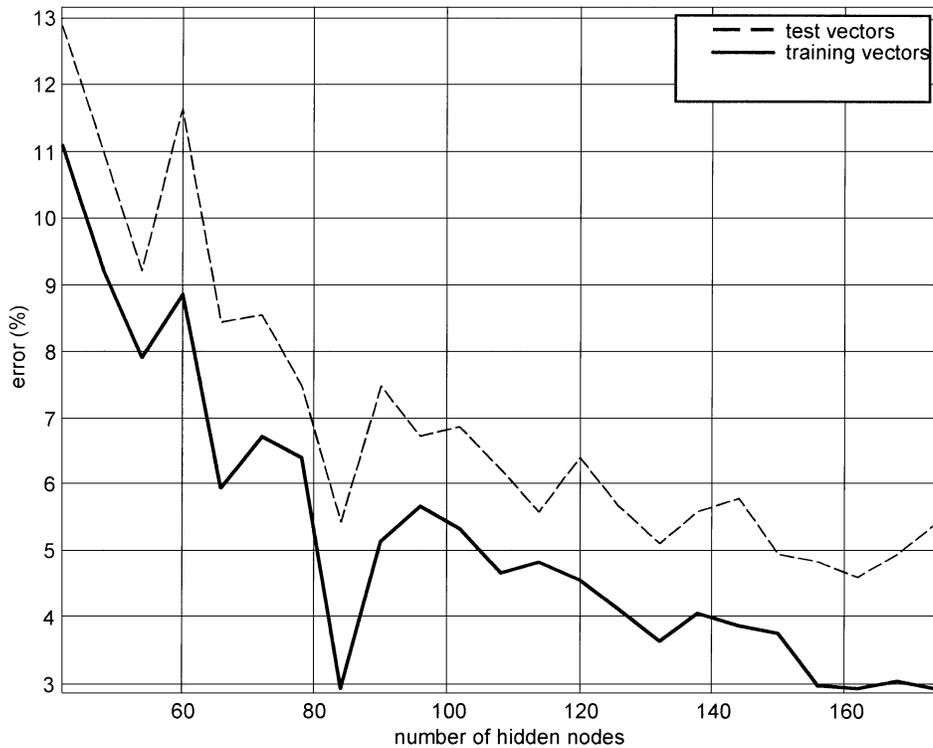
Fig. 6. Classification error as a function of the hidden node number for the CUT in Fig. 5(a).
