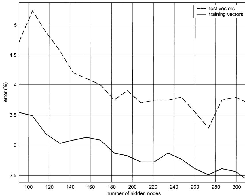
Fig. 3. Classification error as a function of the hidden node number for the Fig. 2 CUT.
