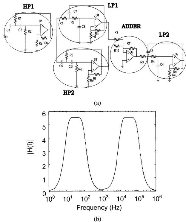
Fig. 4. (a) CUT schematic; (b) CUT transfer function.
